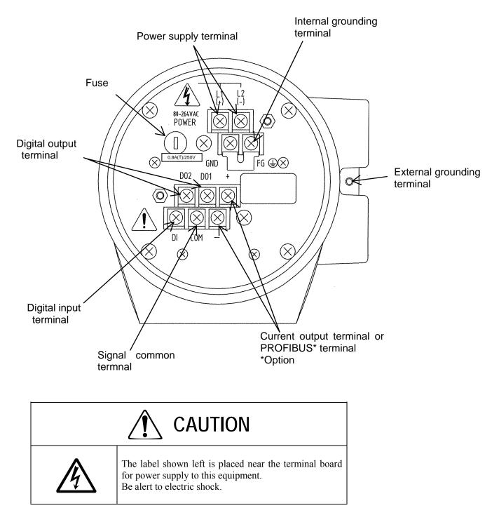
Figure 3.2 Terminal Block Construction of LF546
